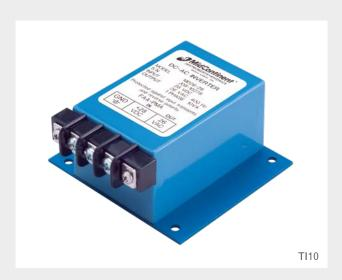
Standing just 1.5 inches tall, the TI10 DC-to-AC Inverter is a small, lightweight inverter designed to provide a reliable source of 26-volt, 400 Hz AC power. The voltage and frequency of its pure sine wave output remains stable regardless of input fluctuations.
